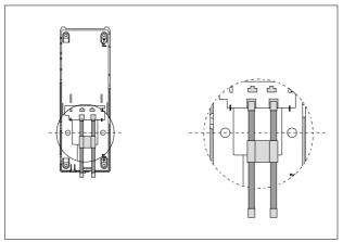
The connection between the junction box and the circuit board of the indoor station is established with the RJ45 connectors included in the scope of supply. Illustration exemplified by AHT/
