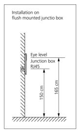
Ideally, an flush mounted junction box should be positioned at the mounting height for the indoor device (display height less 15 cm) (AFS/AFSV/AHT/AHTV/AVP/AHF/ AHFV 870-...).
