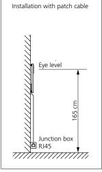
Mounting with Access surface mounting accessory AZA 870-... and patch cable provided on site (AHT/AHTV/AVP/AHF/AHFV 870-...).
