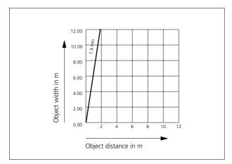
Diagram pickup range Camera ACM 678-... with image pick-up chip 1/3".
