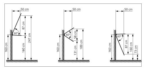
Select the picture excerpt based on the existing mounting situation. The camera's pick-up angle is thus reduced.
