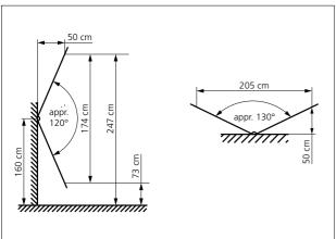
Pick-up angle of the camera module ACM 678-... in full screen mode.
