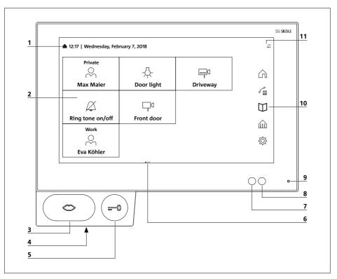
Siedle Axiom is characterised by its generously dimensioned touch-screen. Two buttons are assigned to the basic functions speech and door release. Other functions are actuated at the display.
